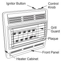
Figure 1 - Vent-Free Gas Heater
